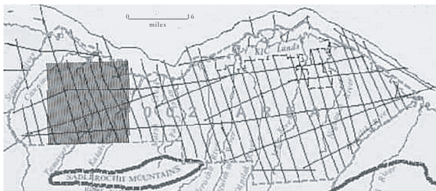
/ Impact lines from 2D seismic exploration in 1984-85 ||| Typical line spacing for 3D seismic exploration, overlaid on part of the coastal plain for comparison
